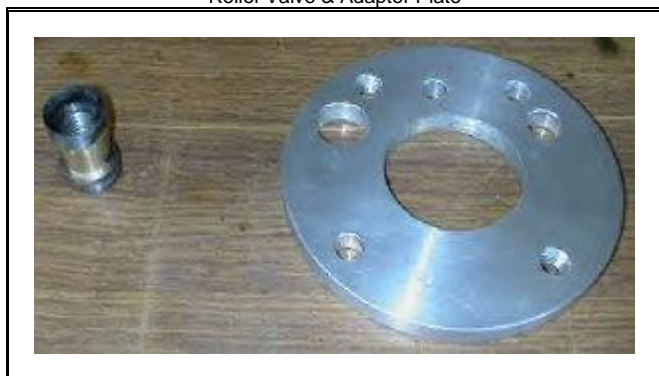
Braze or weld up the holes in the valve
