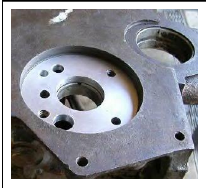
Use Loctite 515 for final assembly
