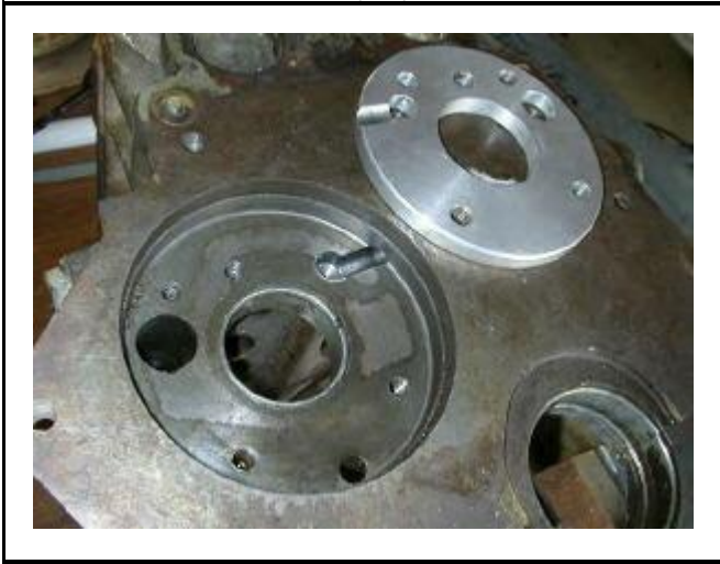
A couple of threaded holes for ease of removal later
