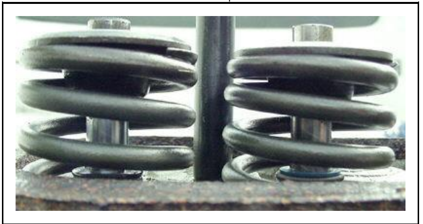
The Viton seal is on the right
